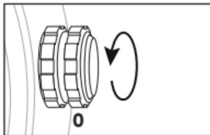
**TO UNSCREW:** Turn the crown anti-clockwise until it turns freely without tension. Gently pull the crown out to the other desired positions for watch setting (see specific operating instructions on the following pages).
